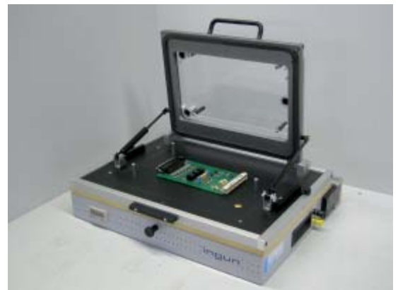
Photos: Vacuum Fixture customized with ZSK 2030-ADP
